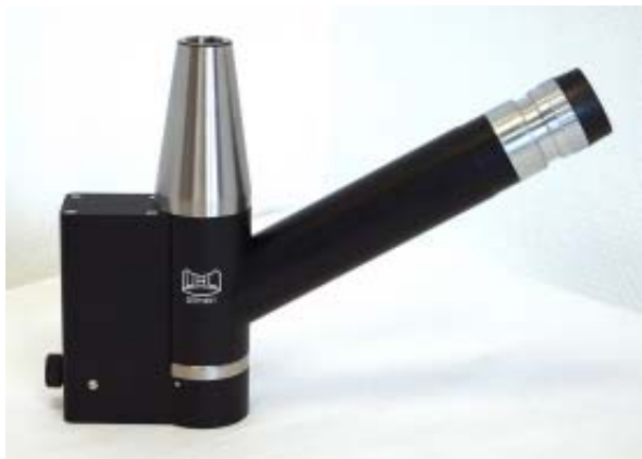
MZM-30A with integrated rechargeable battery for mains power independent operation.
